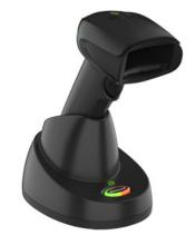
The Xenon XP 1952g-bf wireless scanner offers fast, accurate barcode scanning from up to 10 meters (33 feet) from the base – without the recharge time, expense, and environmental impact of a battery.
